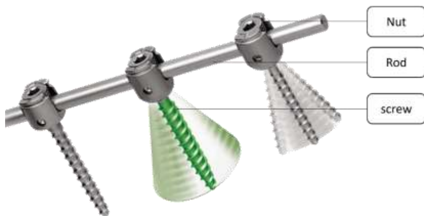
Figure 3 surgery set up with screw, rod and nut
